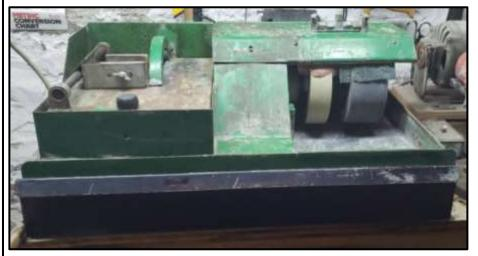
It has a 6" trim saw with a nearly new blade, expandable drum with a large supply of silicon carbide belts, and a 6" polishing wheel that uses interchangeable belts. There are water valves for the drum and the wheel. Asking price \$250. The Kingsley-North catalogue shows a similar machine for \$1350 new.
